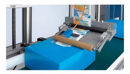
Standard dispensing system: rigid beak with sprung-loaded application roller.
